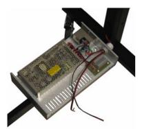
Insert all the power cables through the cable gland and secure the gland locking nut.
