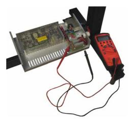
Use DC voltmeter to verify supply voltage
