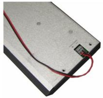
Insert the flat nose screwdriver, carefully twist it to open the contact and insert the stripped cable end. Make sure it contacts properly and that no possible short-circuits exists
