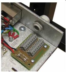
Place the thick washers on the lower beam screw holes, fasten the power supply using the two 5mm size screws with the locking and flat washers in the order shown below. Fasten securely!
