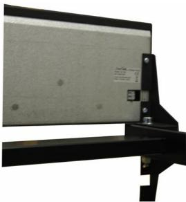
Secure the CH-103 to the brackets using four 4mm screws. Run the power cables through the conduit down to the power supply
