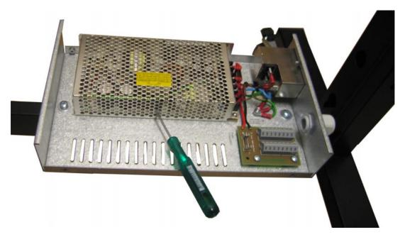
Next, insert the appropriate mains fuse according to the fuse specifications found on the power supply:
