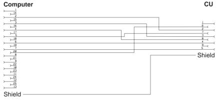
Figure 7.2 - 25 pin connector null-modem serial cable
