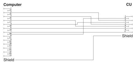
Figure A.1 - 9 to 25 pin null modem cable
